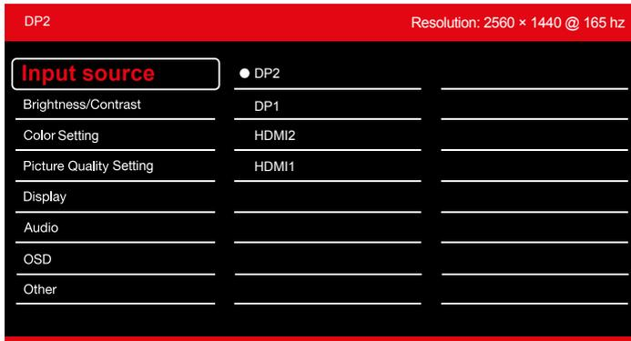
Switch the signal input to DP2, DP1, HDMI2, HDMI1, or have the monitor Auto Select the source.
