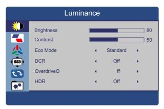
**BRIGHTNESS:** Allows the adjustment of the image brightness, according to ambient light in the room. Value "0–100".
