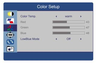
**COLOR TEMPERATURE:** Allows adjustment of the color temperature between the following options: User/Cool/Normal/Warm.
