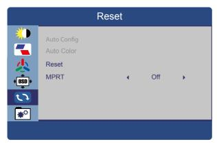
**RESET:** Returns the monitor to its factory default settings. **MPRT:** Allows the MPRT Mode to be turned ON and OFF.
